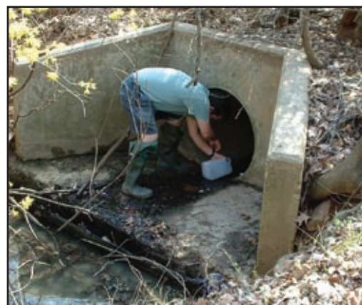
Figure 30: Measuring flow (as volume per time)
