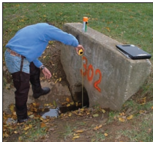
Figure 27: Measuring Outfall Diameter
